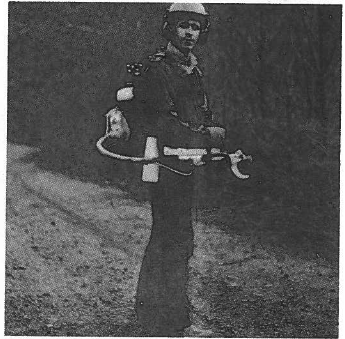
A light backpack motor drives the head through a cable drive. The power-girdling head and drive velcro-straps to the girdler arm, the control handle grip fits comfortably in the hand.
